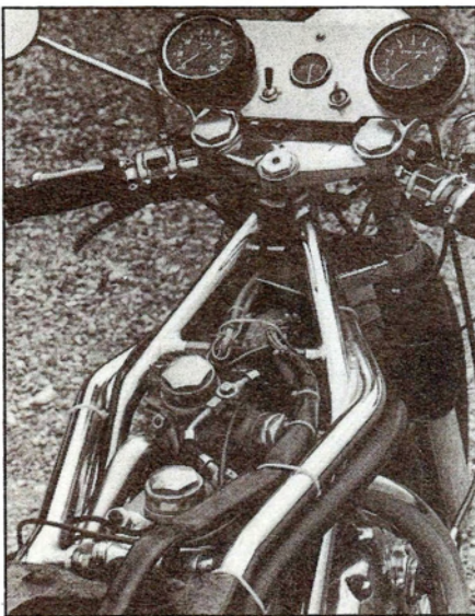
Clearance between the rear cylinder head and the frame tubes is critical
