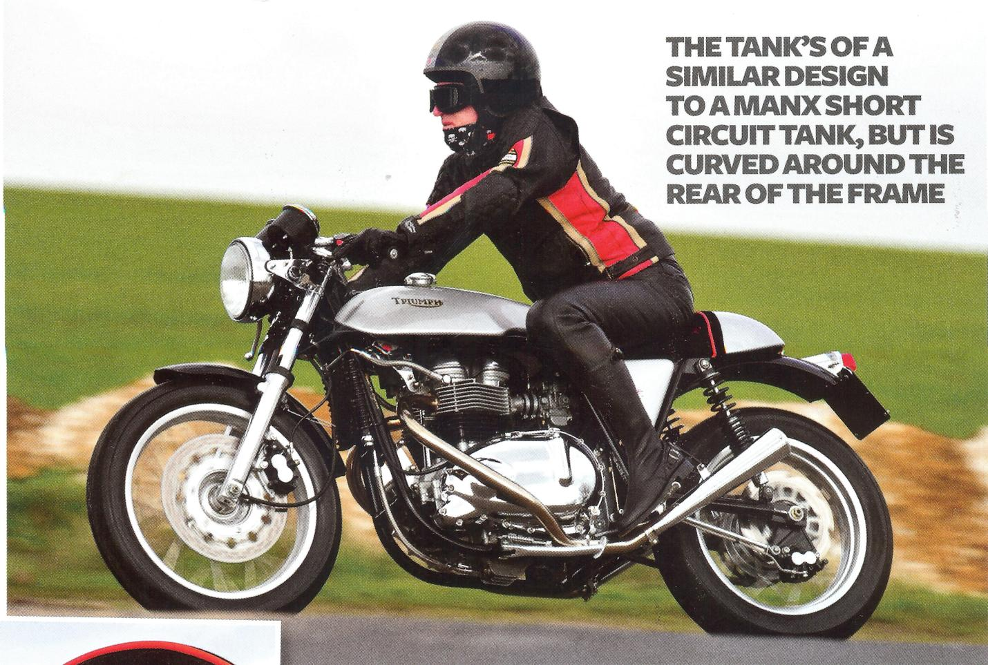
**THE TANK'S OF A SIMILAR DESIGN TO A MANX SHORT CIRCUIT TANK, BUT IS CURVED AROUND THE REAR OF THE FRAME**
