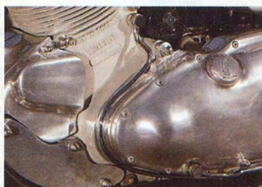
Engine plates were cut with a jig saw
