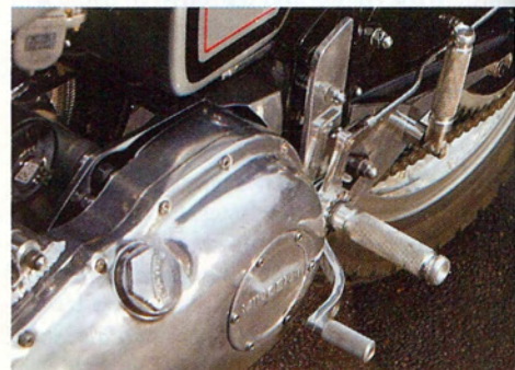
Belt drive is hidden in modified Vincent case
